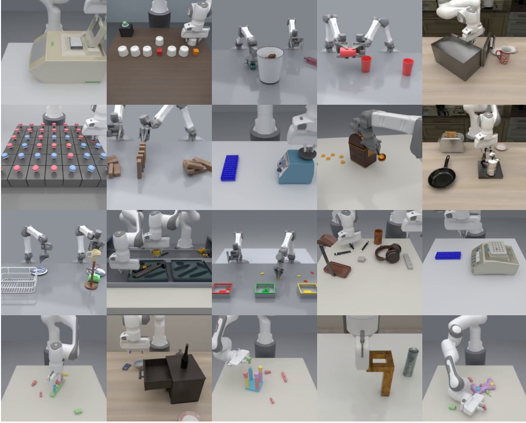
Figure 1: Representative tasks from RoboARCADE. The benchmark includes 22 tasks spanning single and bimanual manipulation, assembly, physical puzzles, and biolab-inspired procedures. This figure shows 20 of them. Tasks require combinations of visual understanding, precise control, memory, and multi-step planning. RoboARCADE supports rendering with Blender for high-fidelity visual observations.
